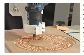
pieces with tools, the movement of which is determined by the machine. In the case of a CNC milling machine, this control is carried out by a computer. As with 3D printing, the template for the workpiece is created using construction software, also known as
