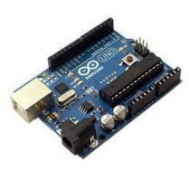
Microcontrollers are essentially simple miniature personal computers (PCs) designed to control small features of a larger component, without a complex front-end operating system (OS). They can be found in a wide range of devices and objects such as vehicles, robots, office machines, mobile radio transceivers and home appliances, among other devices. They can be used for using actuators and sensors.
