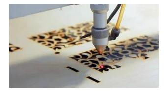
The machine itself is a complex arrangement of partly movable, partly fixed lenses and mirrors, through which a laser beam generated in a laser tube is sent. With the help of these mirrors and lenses, the laser is redirected and treated so
